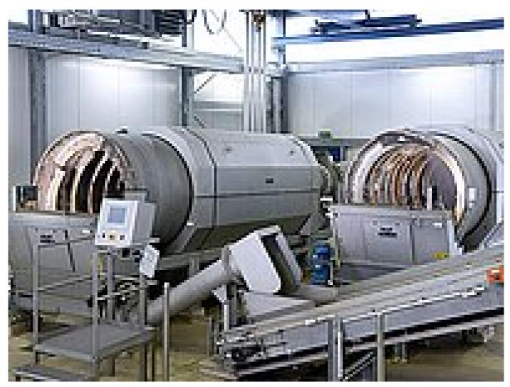
Wash drum for efficient and reliable coarse material separation for septic sludge
