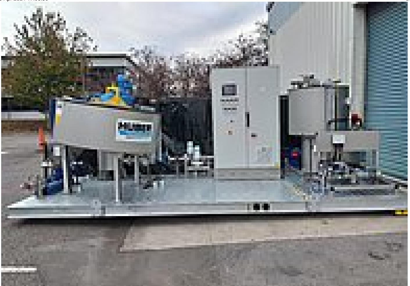
HUBER's Skid mounted sludge thickener S-DISC before delivery to site to Milford Haven
