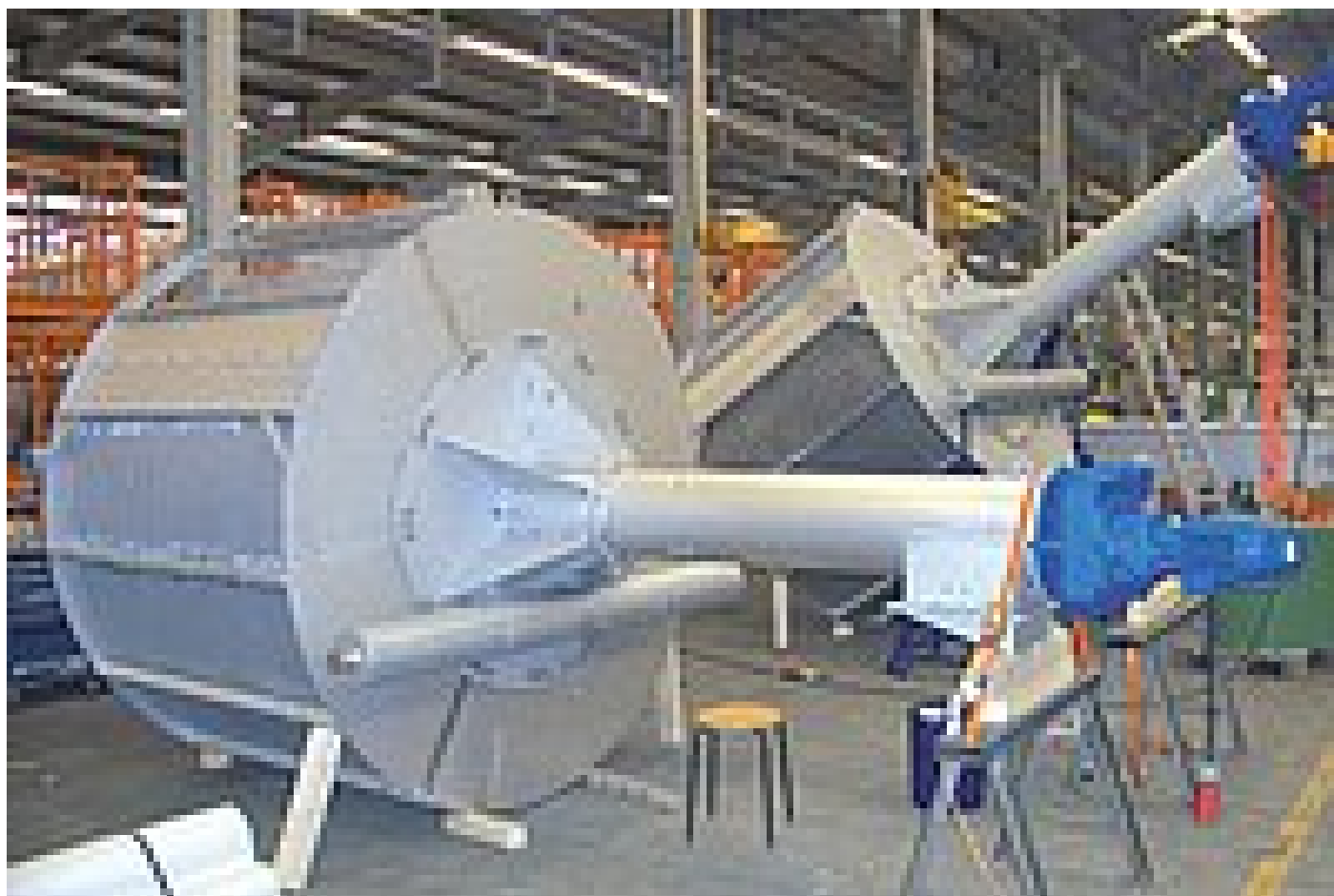
Two of a total of twelve ROTAMAT® Fine Screens Ro 1/2600 supplied for the second construction phase of WWTP Zhuyu
